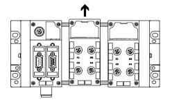
For longer valve terminals, there is an additional mounting bracket (for the CPX terminal) that can be fitted in any module.
