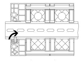
The valve terminal is attached to the H-rail (see arrow A) and then swivelled on the H-rail and secured in place with the clamping component (see arrow B).
