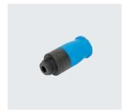
Polymer fitting for easy installation with one hand. Hydrolysis-resistant, FDA-compliant and easy to clean. For pneumatic applications with a temperature range up to 60 °C and a pressure range up to 10 bar.
