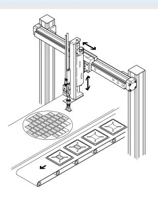
• Pressure sensor SDE5 for suction monitoring when handling small parts, in this case chips.
