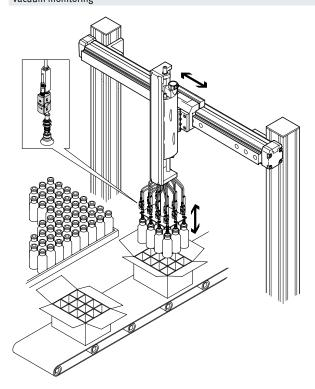
• Pressure sensor SDE5 in combination with a vacuum generator VN for vacuum monitoring when handling bottles
