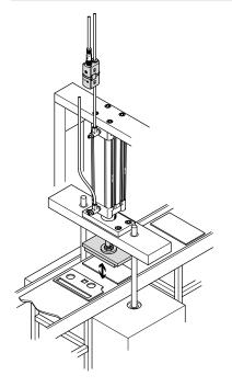
Pressure sensor SDE5 as pressure monitor for the pressing in of punched parts
